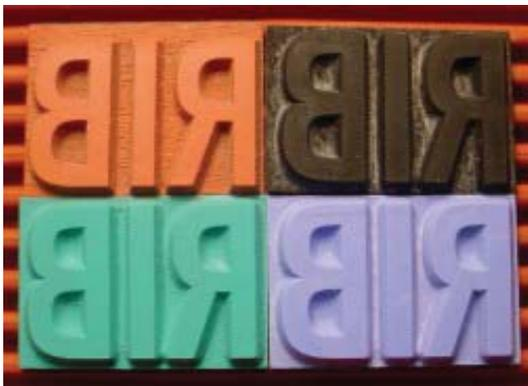
**NATURAL RUBBER:** is best for general purpose use with alcohol and water-based inks. It is available in standard 50 durometer or soft 30 duro.
